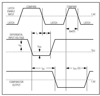
Figure 2. MAX900/MAX902/MAX903 Timing Diagram
