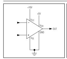
Figure 1A. Separate Analog Supply, Common Ground
