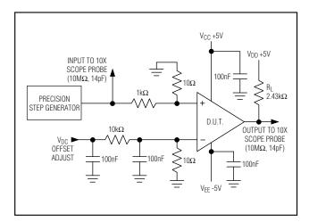
Figure 5. Response-Time Setup
