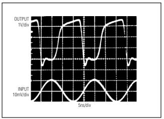
Figure 6. Response to 50MHz Sine Wave
