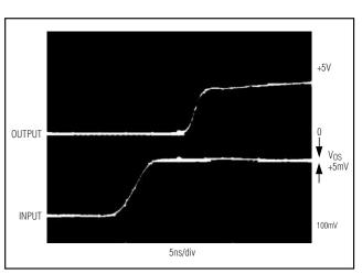
Figure 3. t<sub>pd+</sub> Response Time to 5mV Overdrive
