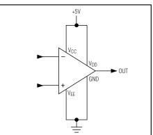
Figure 1B. Single +5V Supply, Common Ground
