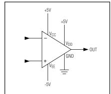
Figure 1C. Split ±5V Supply, Separate Ground
